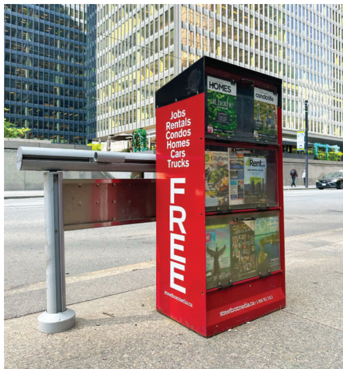
NEWSPAPER CORRALS REDUCE CLUTTER BY PREVENTING MIGRATION OF PUBLICATION BOXES. CORRALS SHOULD BE OF APPROPRIATE SIZE TO MANAGE THE NUMBER OF BOXES.
