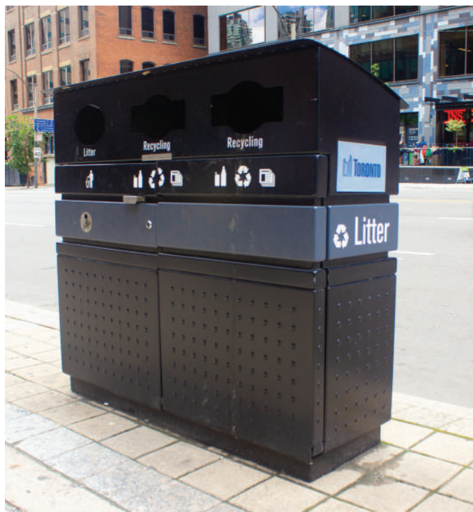
WR4 BINS IN BLACK ELIMINATE THE NEED FOR PEDALS AND FLAPS AND TAKE UP LESS PEDESTRIAN SPACE.
